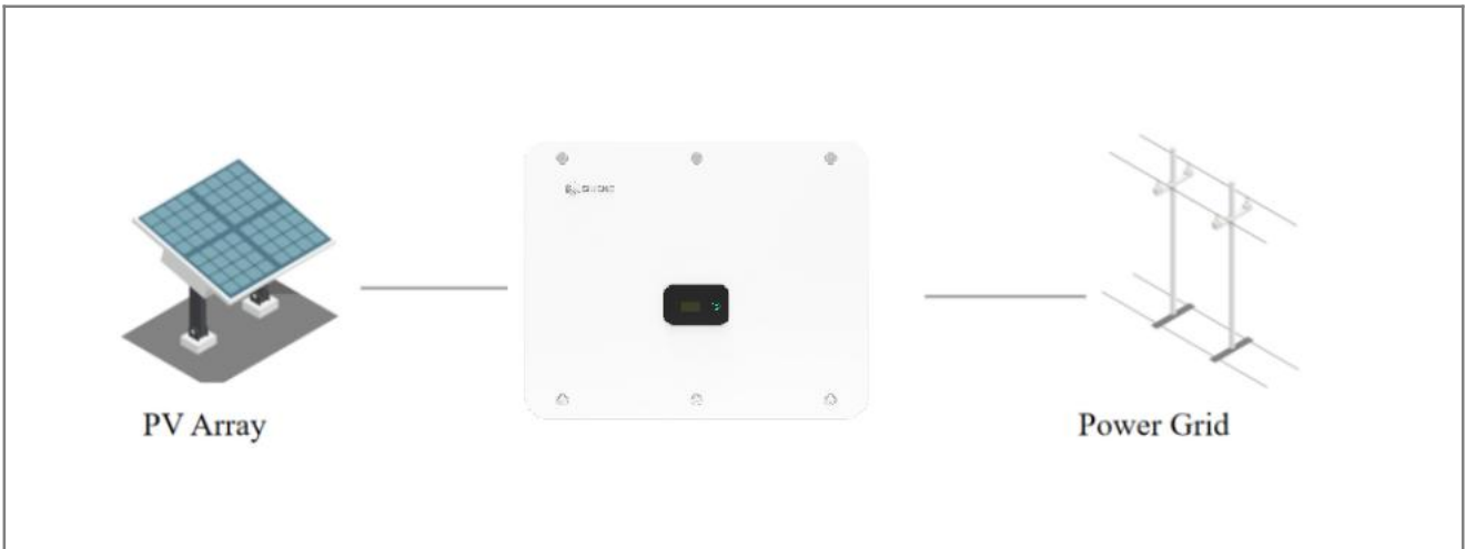
Figure 1-1 Composition of the PV power generation system
