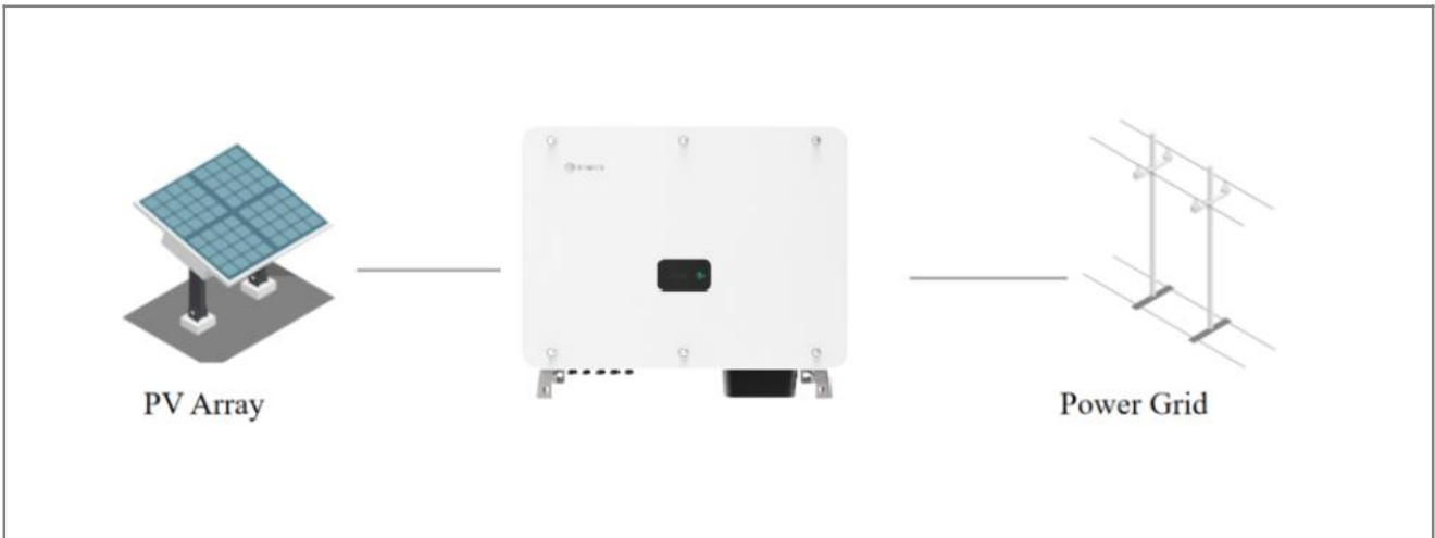
Figure 1-1 Composition of the PV power generation system
