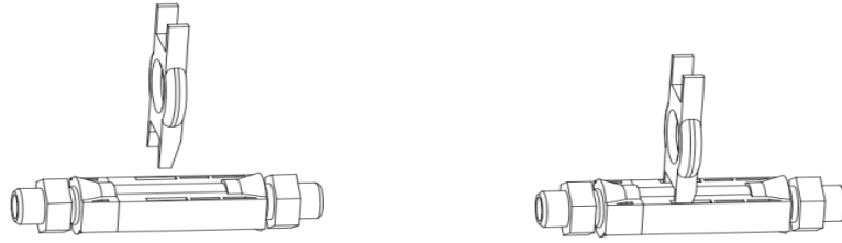
Figure 4-2 Schematic diagram of removing the DC terminal
